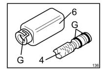
When dismantling parts for washing, regularly check that gaskets [G] are intact and replace them if damaged or dilated.
