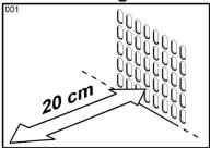
Place the machine on a flat and steady surface.
