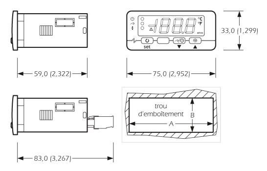
The maximum depth is 89.5 mm whatever the type of connection and refers to models with Faston connections (straight female Faston correctly inserted).
